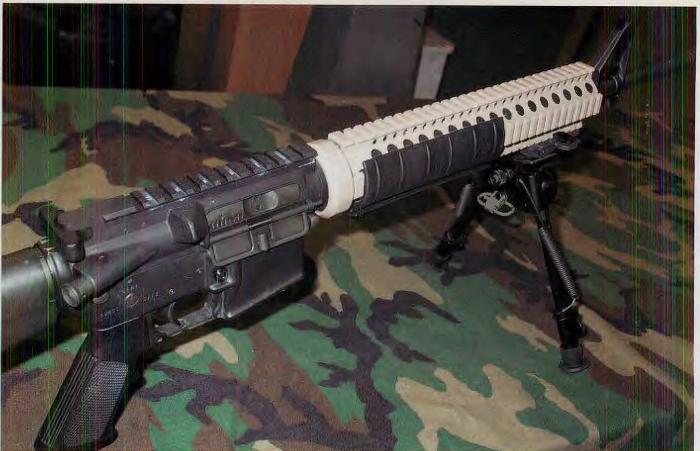
Squad Designated Marksman Rifle features two-stage match trigger, fluted match-grade barrel, choice of handguard rail systems. Rifle has backup detachable carry-handle with iron sights also provided, weighs 8.1 pounds without bipod. Optics, usually an ACOG, will be fitted when rifle is delivered to SDM's unit.
